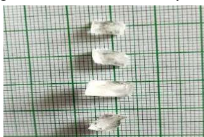
Fig.1 As grown single crystals of CLTC by SSET.
