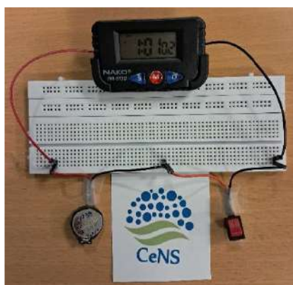
Figure: Fabricated SIB Powering LCD Display
