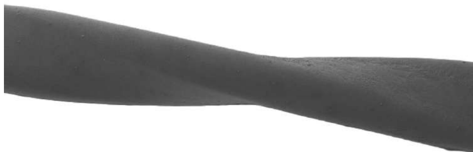
Fig 1: SEM image of flattened and twisted fiber
