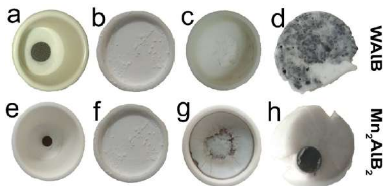
Fig. 1: Modified Molten Salt Shielded Synthesis (MMS 3 ) method for WAIB (a-c) and Mn 2 AlB 2 (e-h) samples. (a,e) Green pellets of WAIB and Mn 2 AlB 2 with salt kept in the alumina crucible. (b,f) Green pellets of WAIB and Mn 2 AlB 2 covered with NaCl-KCl mixture of salt placed inside the alumina crucible. (c,g) Alumina crucible after heating in the box furnace. (d,h) WAIB and Mn 2 AlB 2 sample with solidified salt after heating and breaking the crucible.
