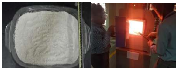
Photographs of Al dross beneficiated \alpha -Al 2 O 3 + MgAl 2 O 4 composite powder and thermal fatigue test
